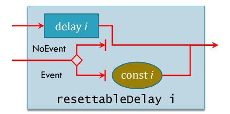
When the event is given, resettableDelay reverts to its starting state.
