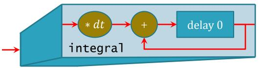
If we could reach in and restart the delay, then integral would behave as if it just started.
