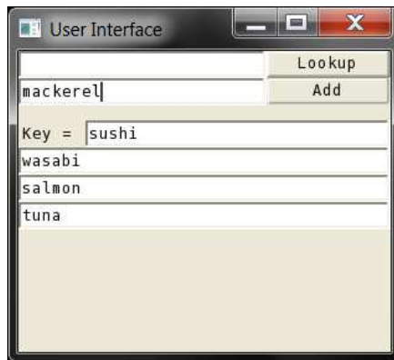
Figure 6.8: The Mind Map GUI. Note that it requires the Haskell Map package to function, as that package provides the insertWith and findWithDefault functions that operate on Maps.
